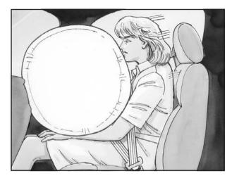
The right front passernger's frontal air bag is in the instrument panel on the passenger's side.
